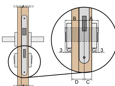
Exemplary calculation of the proper size of patent lock for board and stile door leafs (40 mm) with the thickness of face  $G = 7 \text{ mm}$
